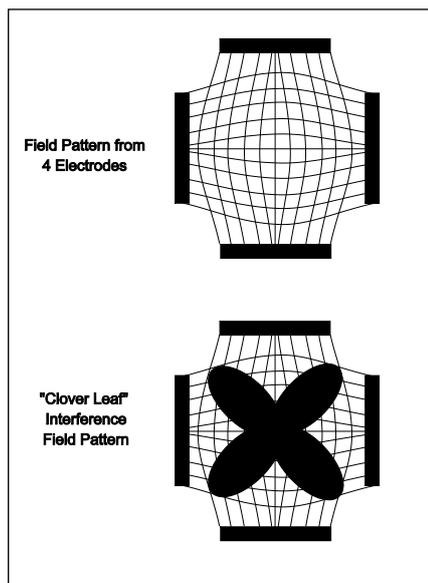
The exact frequency of the resultant beat frequency can be controlled by the input frequencies. If for example, one current was at 4000Hz and its companion current at 3900Hz, the resultant beat frequency would be at 100Hz, carried on a medium frequency 3950Hz amplitude modulated current.
