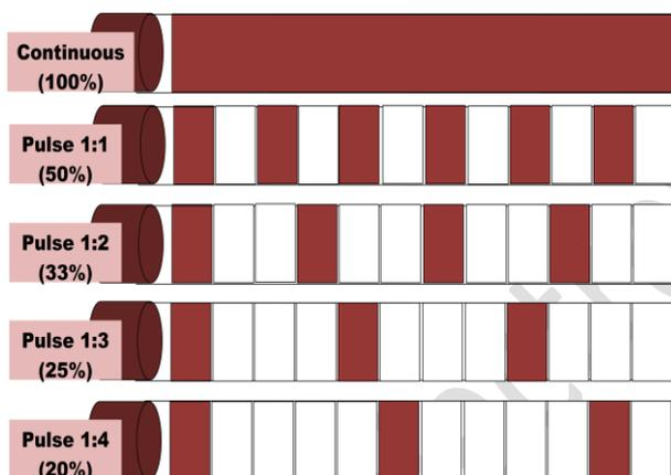
Typical pulse ratios are 1:1 and 1:4 though others are available. In 1:1 mode, the machine offers an output for 2ms followed by 2ms rest. In 1:4 mode, the 2ms output is followed by an 8ms rest period. The adjacent diagram illustrates the effect of varying the pulse ratio.
