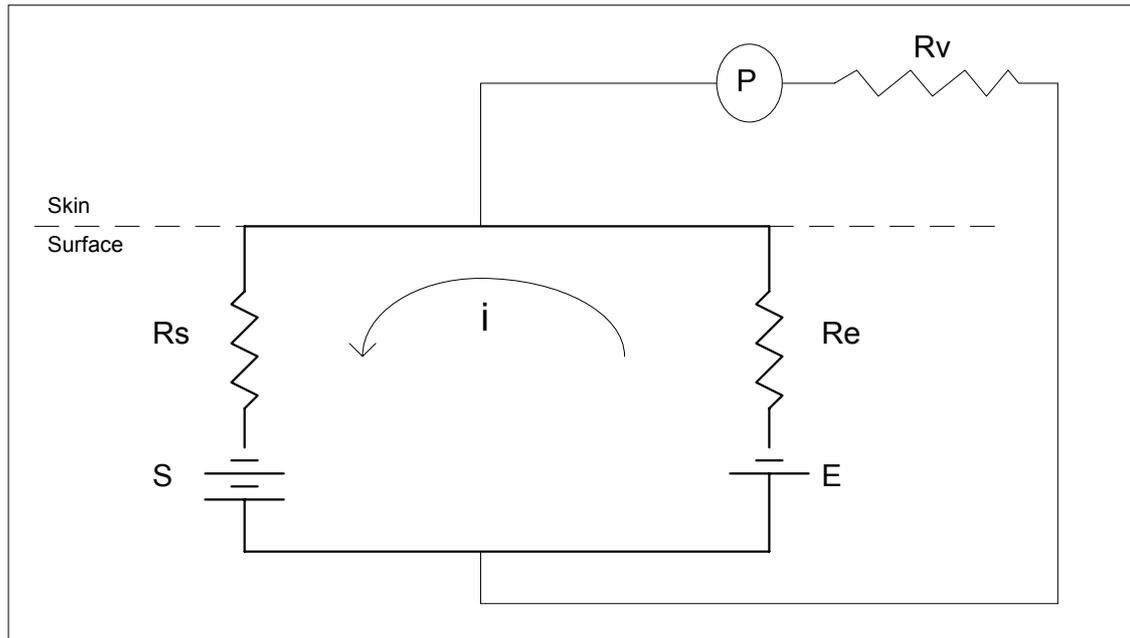
Figure 2.2: Equivalent circuit of Edelberg's Skin Hydration Model
