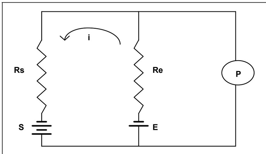
Figure 2.3: Modified Edelberg Skin Hydration Model Circuit
